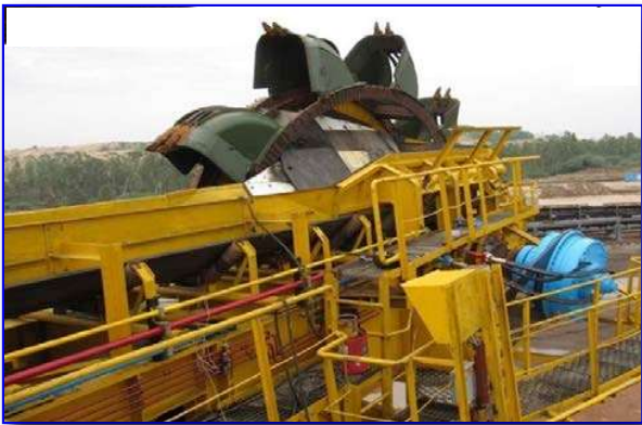
4000 TPH Bucket Wheel Reclaimer Drive
