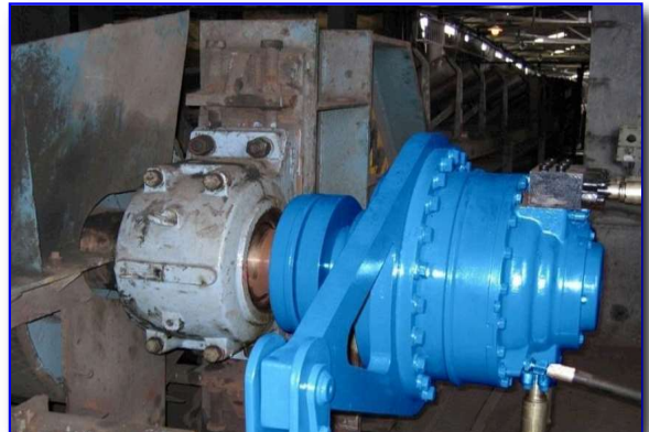
2000 TPH Conveyor Drive Conversion
